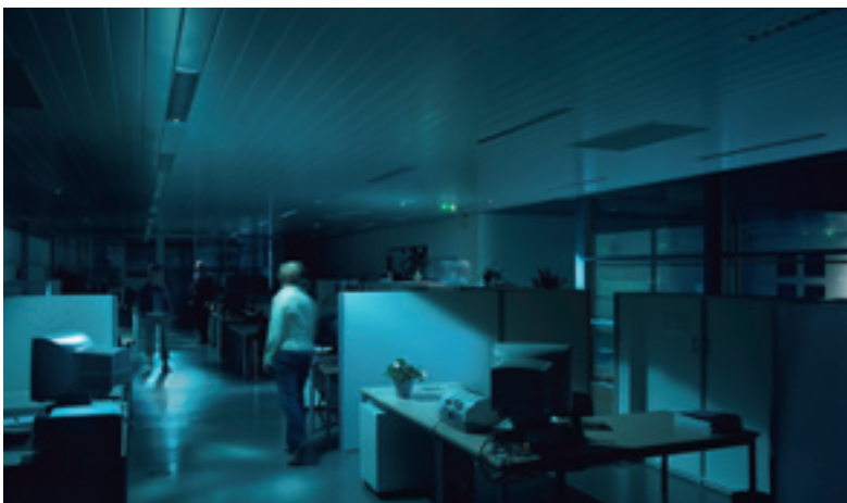
Escape route lighting which, with a mounting height of 3 metres, allows spacings of more than 13,2 metres
