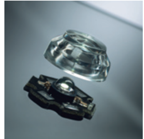
The especially designed lens provides uniform lighting
