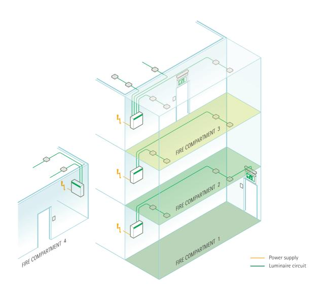
EBS Compact works per fire compartment and thus follows the logic of the building. This makes it easy to plan.
