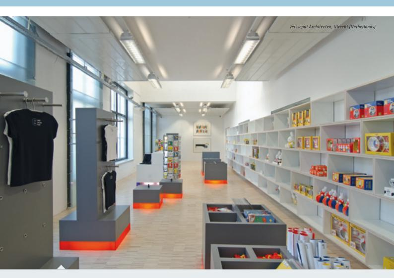
For accurate work or for visual comfort, reflectors with sophisticated aluminium baffles can be chosen to limit the luminance of the luminaires in all directions to less than 1000 cd/m<sup>2</sup>.
