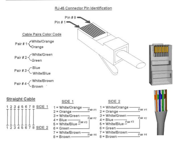
The GreenBus $^{\text{TM}}$  uses the 4 pairs as follows:
