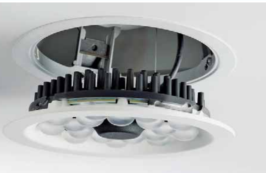
Toolless installation of Flare downlight; the LED module is mounted by means of a twist-and-lock mechanism.
