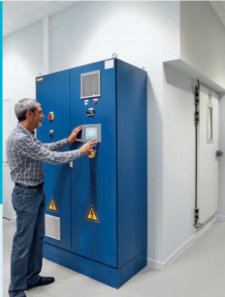
In the climatic chamber, tests can be carried out at temperatures from -20°C to 45°C (including humidity control).
