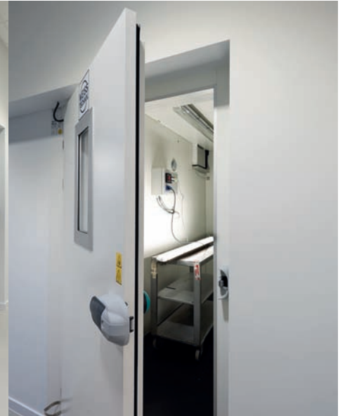
In the climatic chamber, tests can be carried out at temperatures from -20°C to 45°C (including humidity control).
