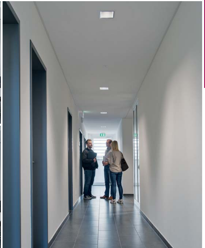
Occupancy detection in the corridors: if no motion is detected for 10 minutes, lighting is dimmed to 20%.
