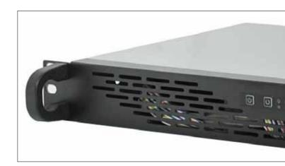
The SSU stores all system settings and parameters, including attributes for zones, luminaires, sensors and push-buttons. Additionally, it maintains multiple set-points, including those for time schedules, occupancy sensor timeouts and peak load features. The SSU also logs historical data regarding the system's operational and energy saving results.
